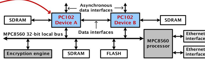
**picoArray MPPA (PC102 device):** Array with 322 processors that communicate over a network of 32-bit unidirectional buses and programmable bus switches.
