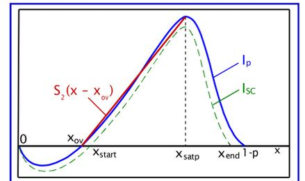
$$E_{SC} = \frac{V_{DD}}{2} (x_{satp} - x_{start}) [(x_{satp} + x_{start} - 2x_{ov}) S_2 - \frac{2C_{gsp} V_{DD}}{\tau} + \frac{V_{DD} k_{sp} \tau}{\alpha_p + 1} [(1-p-x_{satp})^{\alpha_p+1} - (1-p-x_{end})^{\alpha_p+1}] - C_{gsp} V_{DD}^2 (x_{end} - x_{satp})]$$
