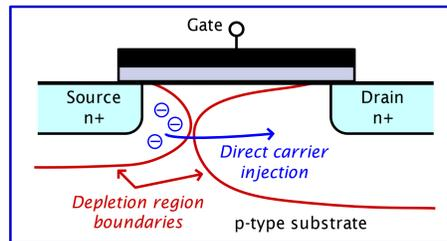
In very short-channel devices, as drain voltage increases, more depletion is performed by the drain bias, and the electric field at the drain penetrates to the source region caused an additional decrease of the barrier at source. This is referred as Drain Induced Barrier Lowering (DIBL) effect. As a result, the device can conduct significant drain current due to an increase of carriers injected from the source.
