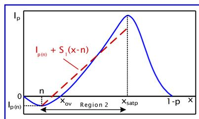
The current slope  $S_1$  is computed by equating the exact PMOS current in the linear region with the approximated one, at  $x = (1-p)/2$ . After that, the output voltage waveform in region 2, is described by:
