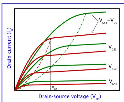
The modeling of mobility degradation and velocity saturation effects is achieved by employing the velocity saturation index ( $\alpha$ ) to describe the power laws featuring the drain current and the drain-source saturation voltage:
