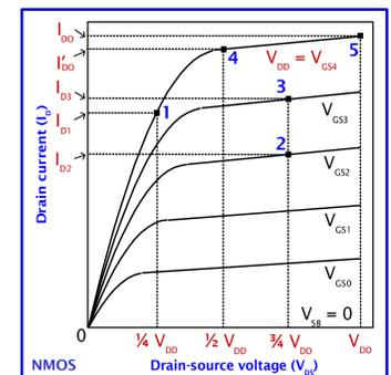
Velocity saturation index is extracted from  $I_{Dsat}$  expression by using the fitting points 2 and 3.  $V_{DO}$  is computed by combining  $I_{Dtri}$  and  $V_{DO}$  expressions and using the fitting point 1:
