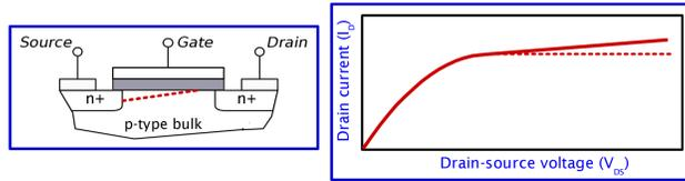
When the device operates in saturation and the drain voltage increases, the uninverted region at the vicinity of the drain (pinch-off region) expands toward the source, shortening the length of the channel region. Due to the fact that resistance is proportional to length, shortening the channel decreases its resistance, causing an increase in current with increase in drain bias for a device operating in saturation.
